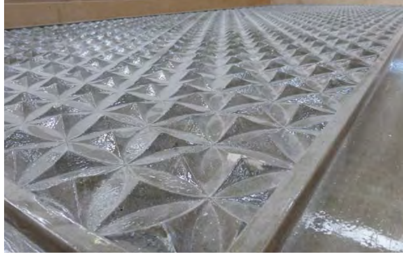
One of the concrete moulds used for GRC panel manufacture.
